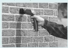
Using the wireless feature of the Sensus AutoGun, inside meter remote TouchPads or underground meters equipped with TouchRead PitLid (TR/PL) units are read in less than two seconds. (below and right)
